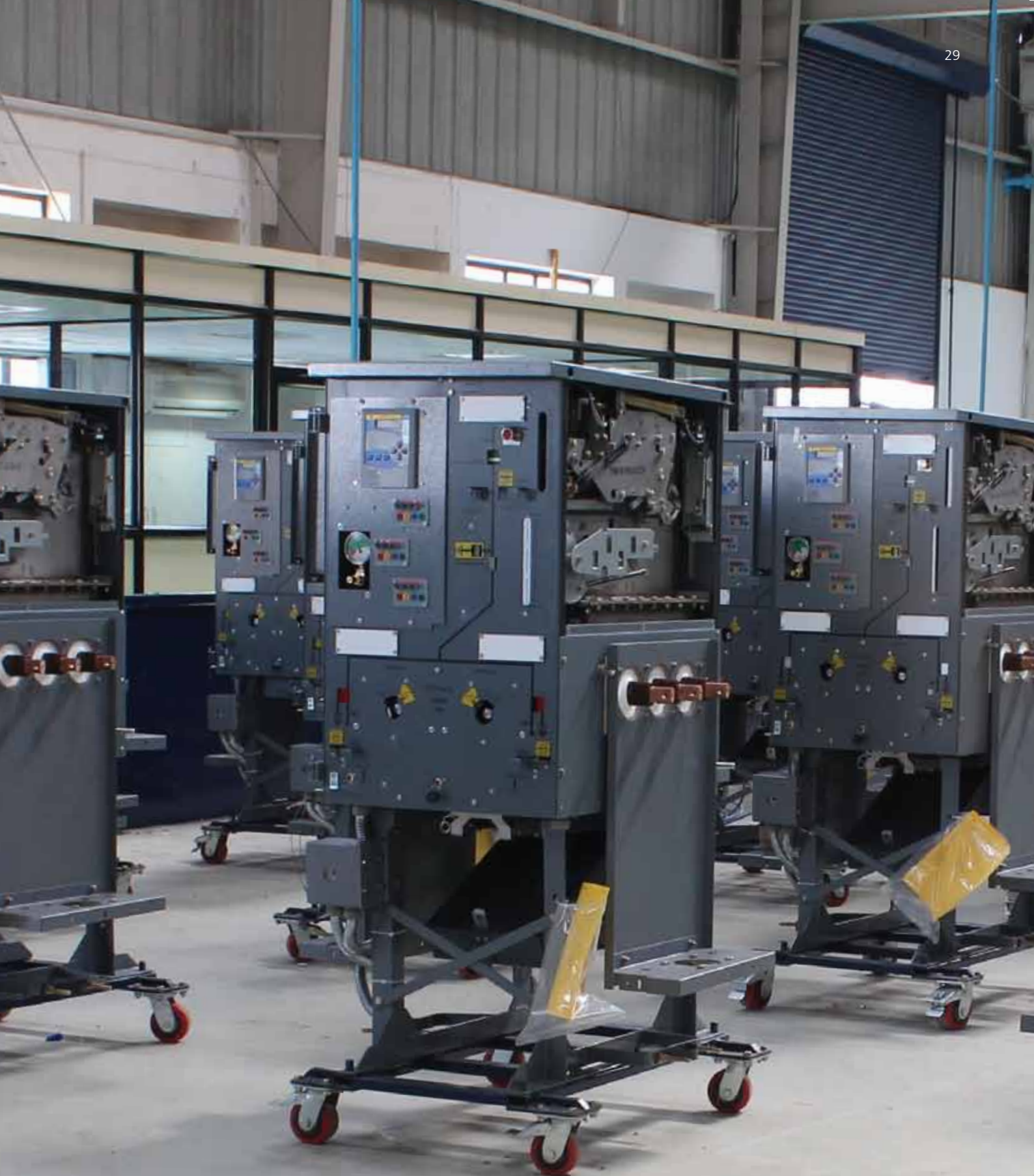
Sabre ring main unit production, Lucy Electric India (Private) Ltd
